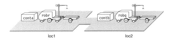
move(r, l, l');; robot r at location l moves to a connected location l'precond: at(r, l), adjacent(l, l')effects: at(r, l'),  $\neg$  at(r, l)
