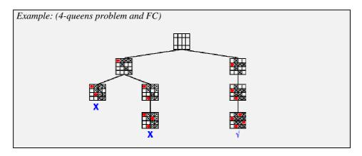
Forward checking detects the inconsistency earlier than chronological backtracking and thus it reduces the search tree and (hopefully) the overall amount of work done. But it should be noted that forward checking does more work when an instantiated variable is added to the current partial assignment. Nevertheless, forward checking is still almost always a better choice than simple backtracking.
