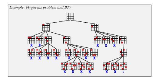
As we demonstrated with backjumping and backmarking strategies, the BT algorithm can be easily extended to backtrack to the conflicting variable and, thus, to incorporate some form of look-back scheme or intelligent backtracking. Nevertheless, this adds some additional expenses to the algorithm and it seems that preventing possible future conflicts is more reasonable than recovering from them.
