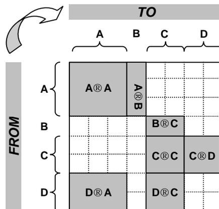
Fig. 2. A transition constraint expressed as a table of compatible transitions (shadow regions).
