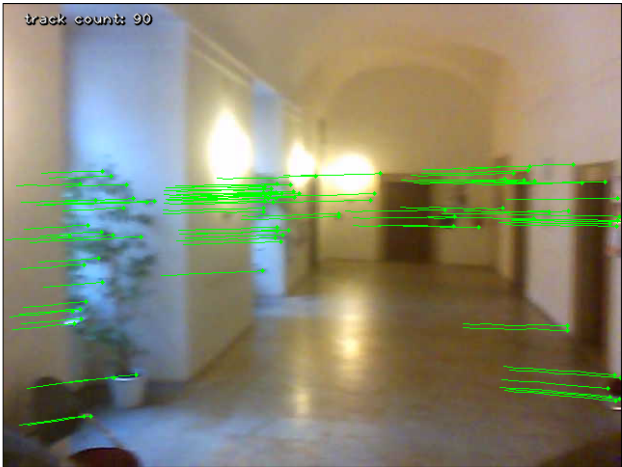
Figure 2: Frame recorded by drone with dominant rotation. Keypoints tracked by Lukas-Kanade method are show in green together with history of tracked positions of each keypoints.
