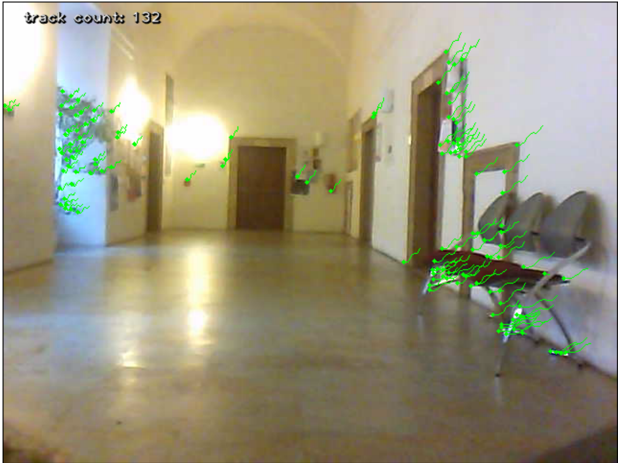
Figure 3: Frame recorded by drone with dominant translation. Keypoints tracked by Lukas-Kanade method are shown in green together with history of tracked positions of each keypoint.
