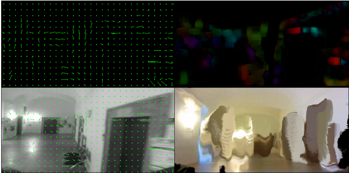
Figure 1: Top-left: dense flow visualised on black background. Bottom-left: dense flow visualised on original video frame. Note the noise around the doors. Top-right: HSV visualisation of the same flow. Bottom-right: Previous frame transformed according to the flow.
